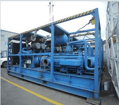
High speed high volume de-oiling/flushing pump suitable for pipeline decommissioning
