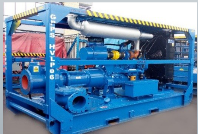
Rig-safe multistage centrifugal pump delivering up to 14.3barg and 19.8bbl./min. discharge
