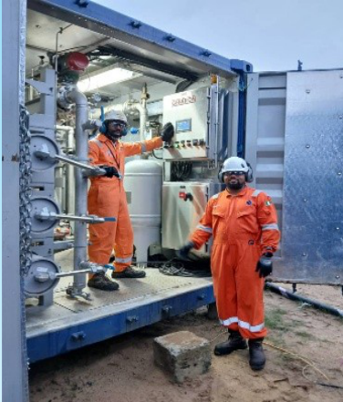
Nitrogen membrane with the operators on site in a nitrogen supply project
