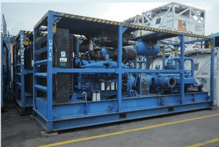
Rig-safe multistage centrifugal pump delivering up to 45barg and 78bbl./min. discharge
