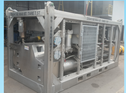
Hydraulic unit with max. inlet pressure of 1 bar & outlet pressure of 25 bar at 174 GPM
