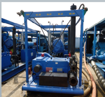
High pressure moderate volume de-oiling/flushing pump suitable for pipeline decommissioning
