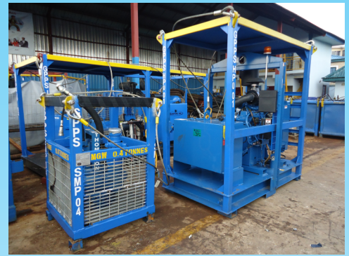
Hydraulic-driven submersible pump delivering up to 48bbl./min & head of 39m with powerpack
