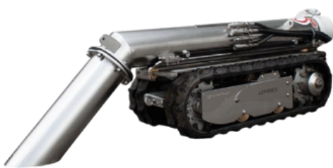
Atex Zone 0 Certified Robot with Antistatic Anti-oil Chemical Resistant Rubber Tracks and Suction Hose 100[mm] (4") with quick Couplings for super automated tank cleaning
