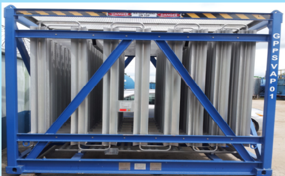
Ambient Vaporiser is used to convert nitrogen to gaseous and delivering output pressures up to 40 bar (working) or 57.2 bar (testing)
