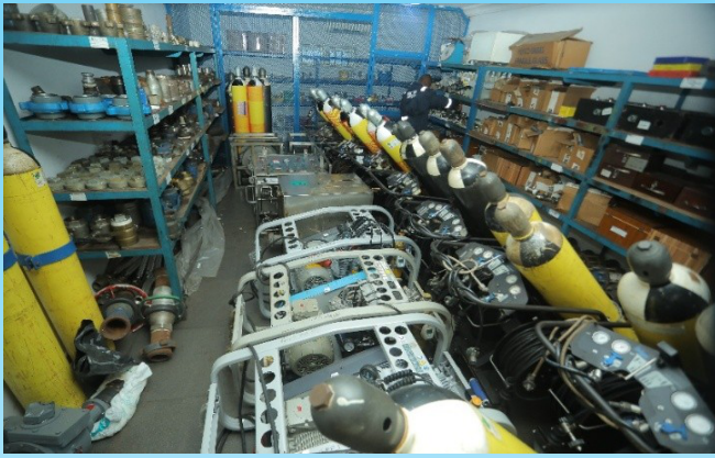
SETS OF TANK CLEANING AIR-OPERATED VACUUM PUMP CAPABLE OF SUCKING SLURRIES/SLUDGE FROM UP TO 50M & DELIVERS TO 1000M AT FLOW RATE OF UP TO 40CMH AND ACCESSORIES IN OUR PORT HARCOURT BASE
