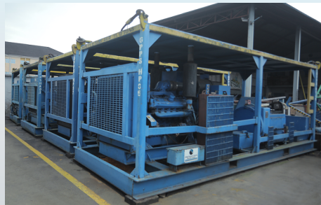
Rig-safe quintuplex plunger pump delivering up to 113barg & 12.9bbl./min.
