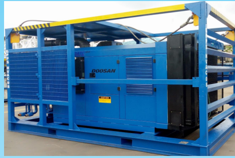
High volume air compressor with up to 24 barg & 1200 SCFM discharge
