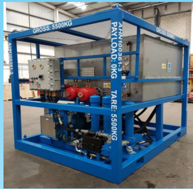
Diesel flushing unit with filtration degree of 0.8-3 microns filters & flow rate of 0.8-35 GPM
