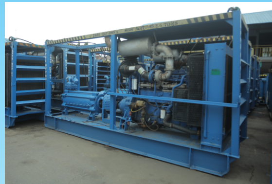
A high velocity flushing pump used for high-volume long-distance pipelines and vessels
