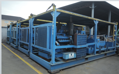
High pressure moderate volume de-oiling/flushing pump suitable for pipeline decommissioning
