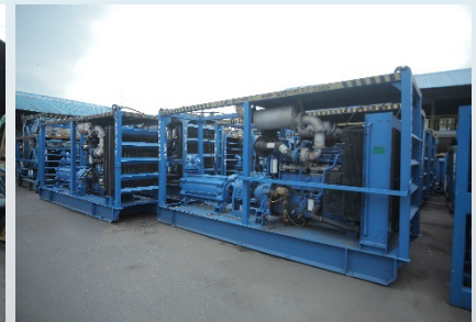
Rig-safe multistage centrifugal pump delivering up to 34barg and 46bbl./min. discharge
