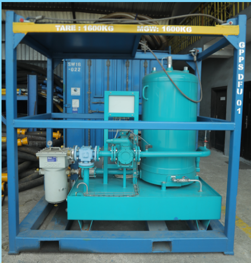
Mineral oil flushing unit with 2-25 micron filters & 422 GPM at 31 bar & oil viscosity of class 32
