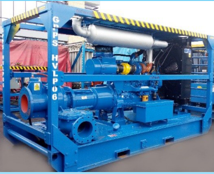
High volume high lift de-oiling/flushing pump suitable for condensate transfer & pipeline decommissioning
