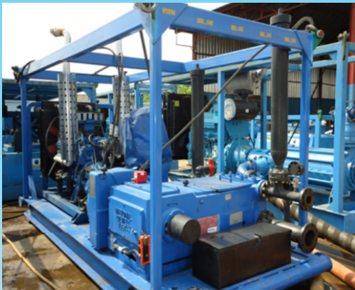
Rig-safe triplex plunger pump delivering up to 113barg & 7.7bbl./min
