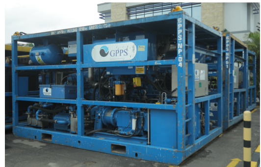
Rig-safe liquid nitrogen pump for nitrogen leak test delivering up to 10kpsi & 180 kSCFH
