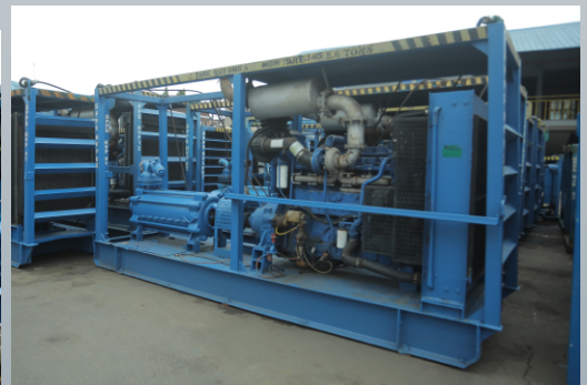
High speed medium volume de-oiling/flushing pump suitable for pipeline decommissioning
