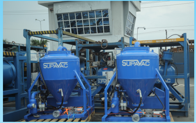
SETS OF TANK CLEANING AIR-OPERATED VACUUM PUMP CAPABLE OF SUCKING SLURRIES/SLUDGE FROM UP TO 50M & DELIVERS TO 1000M AT FLOW RATE OF UP TO 40CMH AND ACCESSORIES IN OUR PORT HARCOURT BASE
